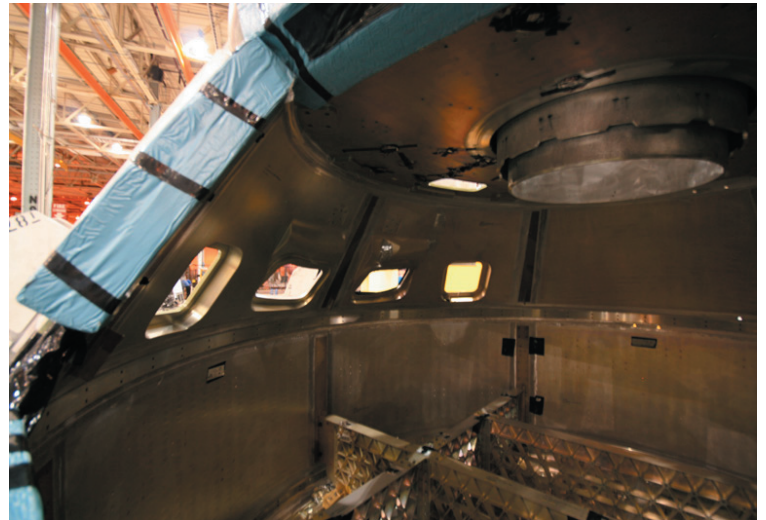
Peering into Orion GTA crew cabin through the crew hatch toward astronaut windows at left and tunnel at top. Credit: Ken Kremer
