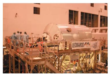
'Leonardo' Multi-purpose logistics module (MPLM) inside the Space Station Processing Facility at KSC is loaded with 16 science and equipment storage racks and platforms. Credit: Ken Kremer
