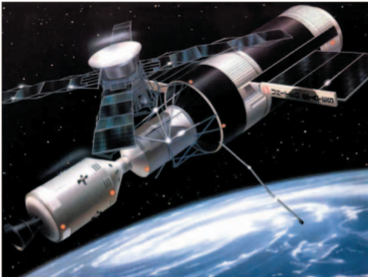
Skylab with docked Apollo Command and Service Modules and Apollo Telescope Mount with its four solar arrays.
