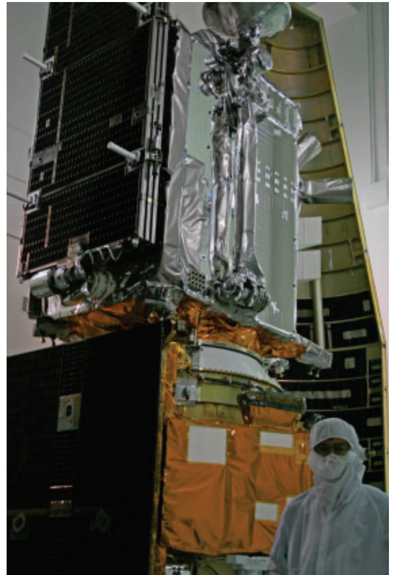
Solar arrays power science for LRO (top, left) and LCROSS (bottom, left) in the "Clean Room" at Astrotech Space Operations Facility nearby Kennedy Space Center: Ken Kremer adjacent to LCROSS panel with 9 science instruments (gold color) which reside just above, left of my garbed head. Payload fairing in background. One month before lunar blast-off on June 18, 2009. Read my mission reports online at The Planetary Society.
